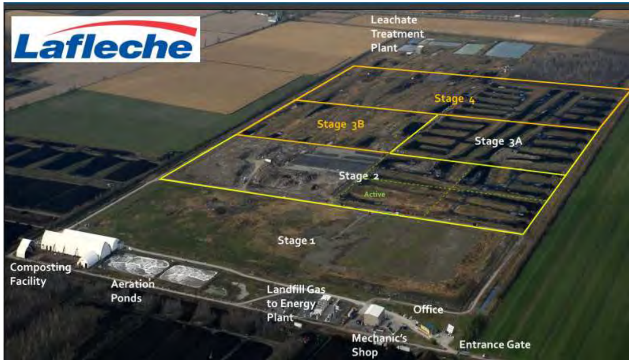
Figure 2: Layout of Eastern Ontario Waste Handling Facility
